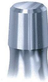
Undamaged stem taper
